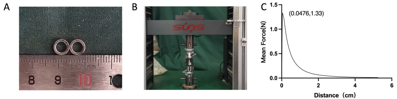
Fig. 4. The magnetic ring used in surgery. (A) Physical representation of the anastomotic magnetic rings used during surgery. (B) A universal testing machine (Shenzhen Sansi Zongheng Technology Co., Ltd., Shenzhen, China) was used to measure the actual attraction force between the magnetic rings. (C) The mean magnetic force-distance curve shows a mean peak force of 1.33 N.
