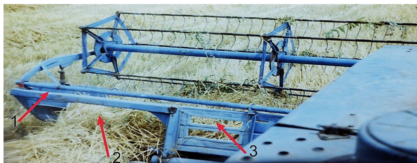
Figure 6. View of the windrower from the tractor driver's seat with the tractor moving forward: 1—left divider; 2—unloading window; 3—viewing window.
