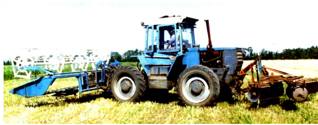
Figure 1. Harvesting unit with reversible tractor movement.
