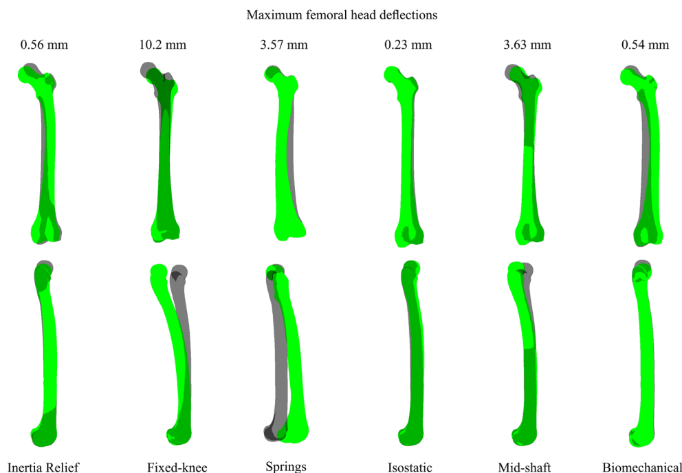
Figure 4. Deflected femur (green) in posterior (top row) and lateral (bottom row) views overlaid on neutral (undeformed) femur geometry (grey) during midstance. All deflections are uniformly scaled tenfold for clarity.
