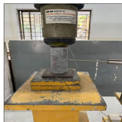
d. UCS test on a rock specimen
