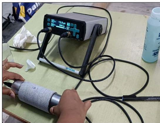
a. UPV test on a rock specimen
