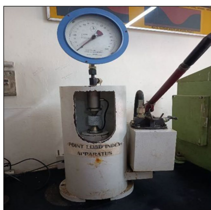
c. Point load test on a rock specimen
