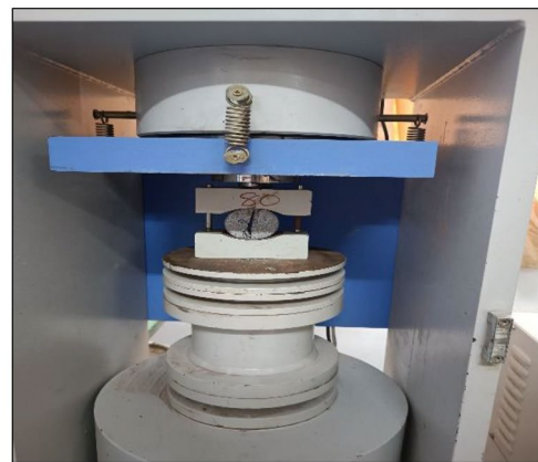
b. BTS test on a rock specimen
