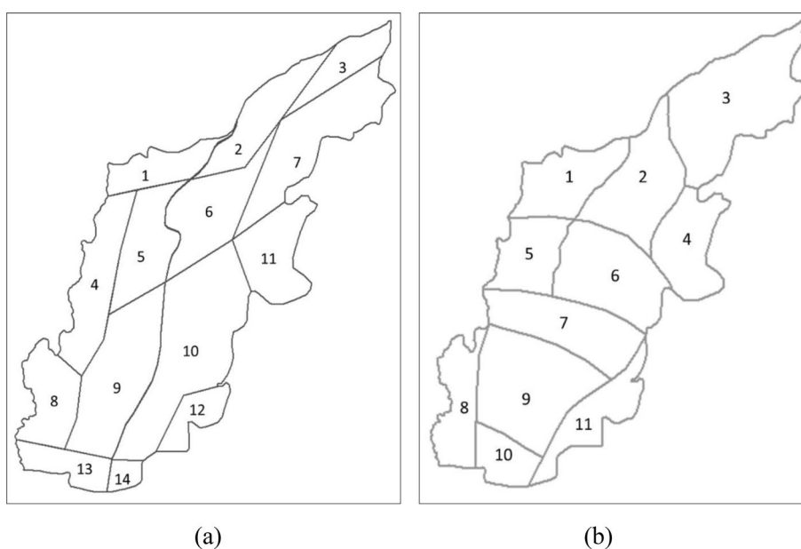
Figure 4. Hydrogeological parameter zoning map: (a) hydraulic conductivity; (b) precipitation infiltration coefficient.
