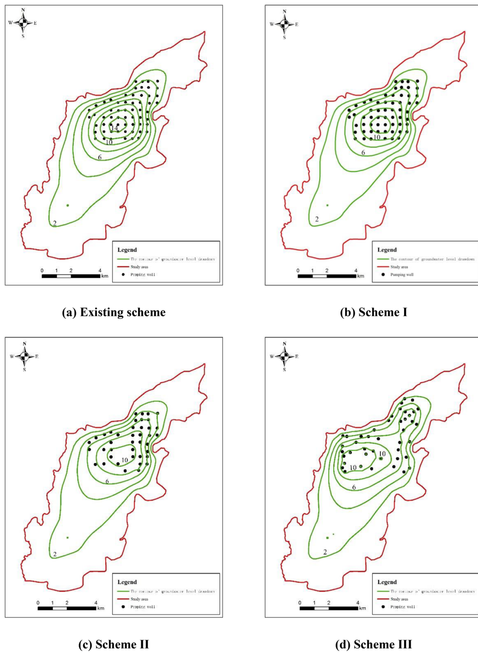
Figure 15. Contour maps of groundwater level drawdown after three months of water supply.
