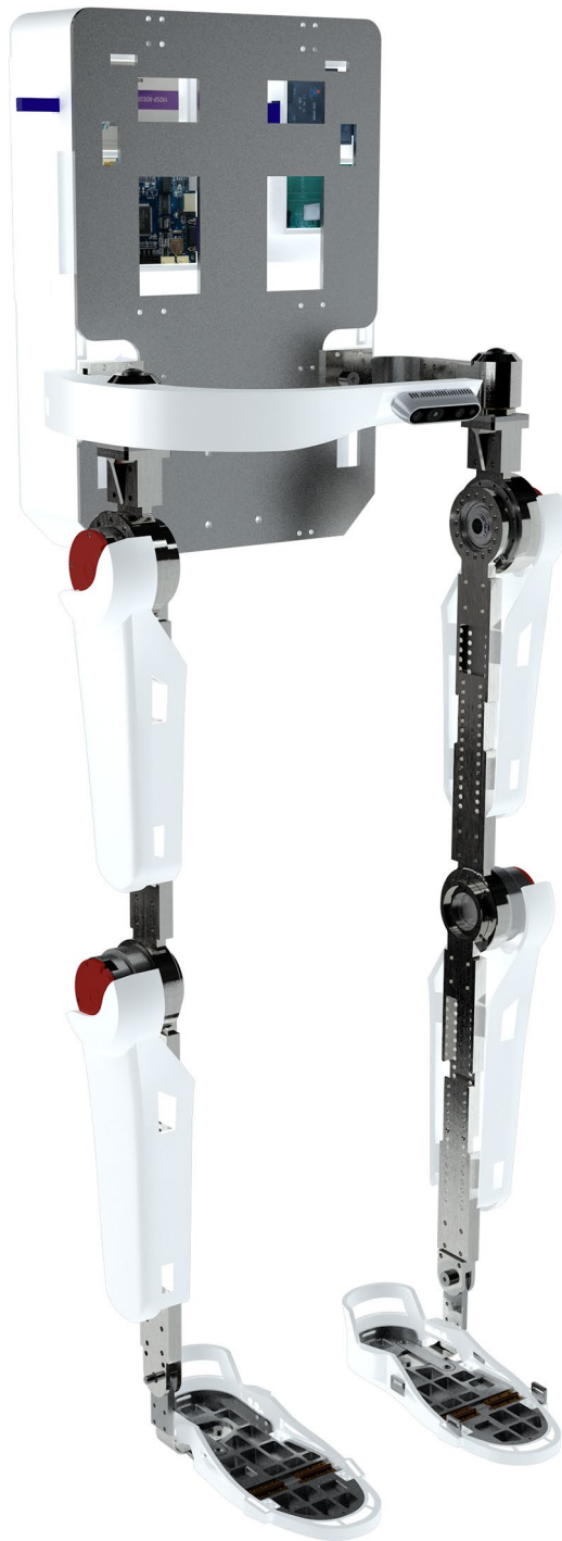
Figure 8. Mechanical structure of lower limb exoskeleton rehabilitation robot.
