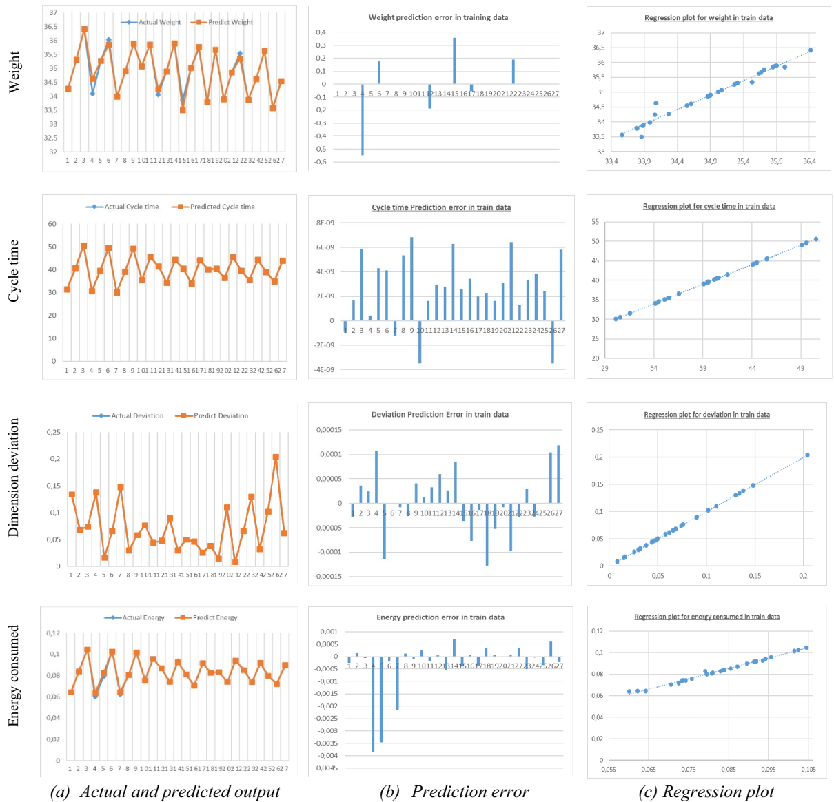
Figure 5. Results plots of ANN model developed for process mapping of part injection molding in training data.
