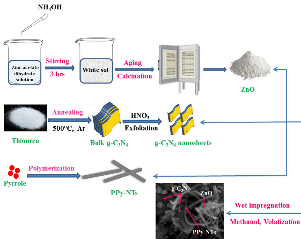
Figure 1. Schematic illustration of ternary ZnO/PPy-NTs/g-C 3 N 4 fabrication procedure.
