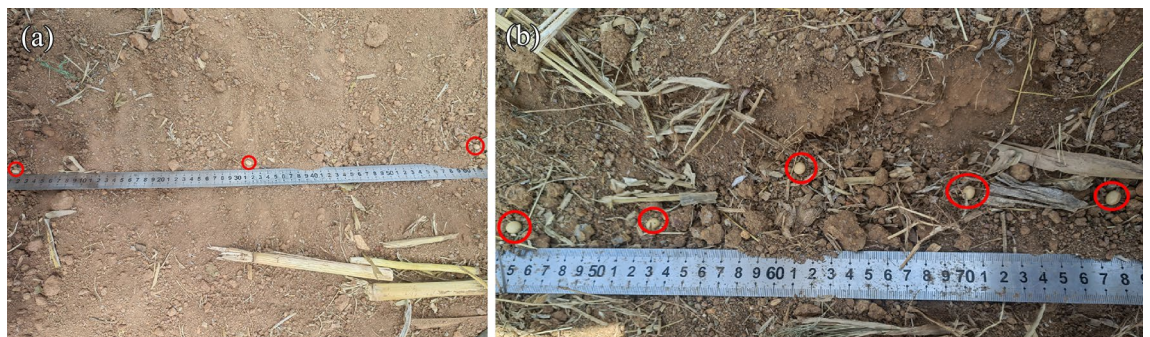
Figure 13. Comparison of seeding quality. (a) Seeding by spoon-type seeder; (b) seeding by shaftless spiral seed discharge and seed delivery device.
