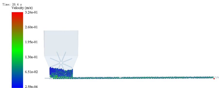
Figure 10. Simulation model of shaftless spiral seed discharge and seed delivery device.
