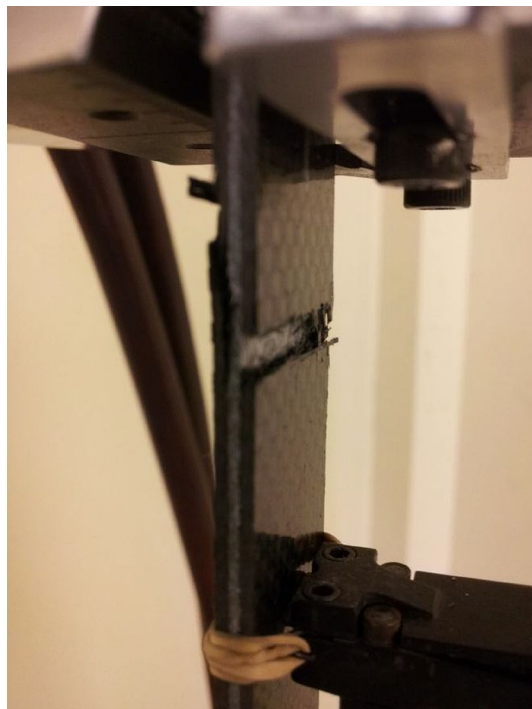
Figure 4. Failure of 3D/67 under tensile loading, Specimen size 254 mm × 25 mm × 4 mm.
