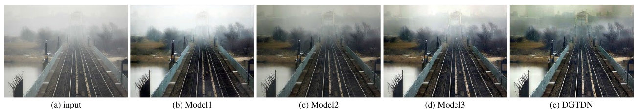
Figure 8. Visual results of different model configurations and the proposed method. The dehazed result obtained by other different models often retains haze or color distortion. The proposed method can remove haze more completely and obtain a more natural dehazing result.
