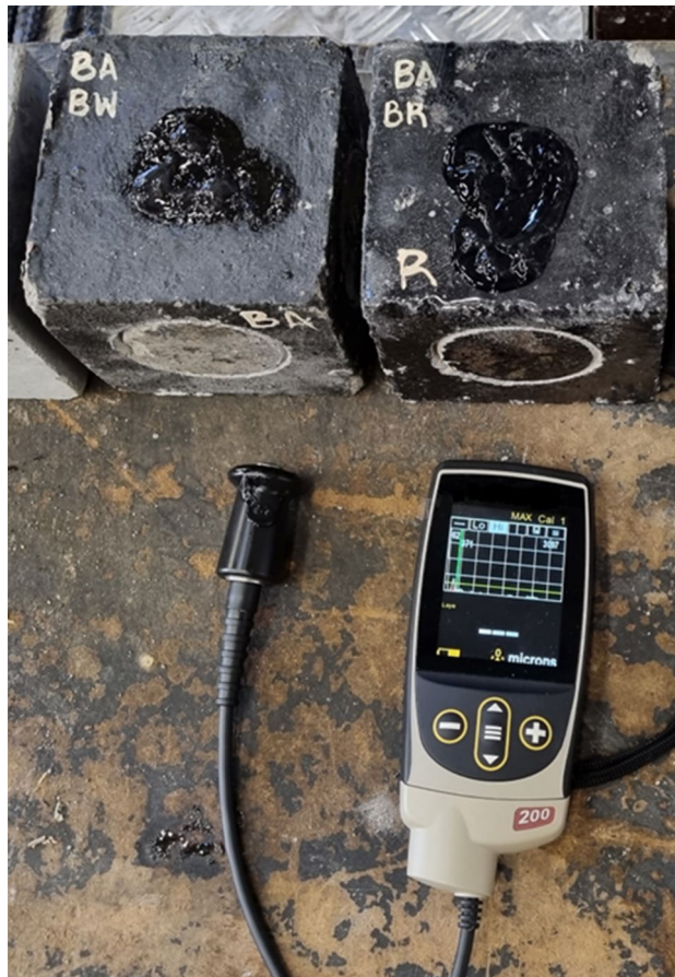
Figure 3. Measurement of coating material thickness.
