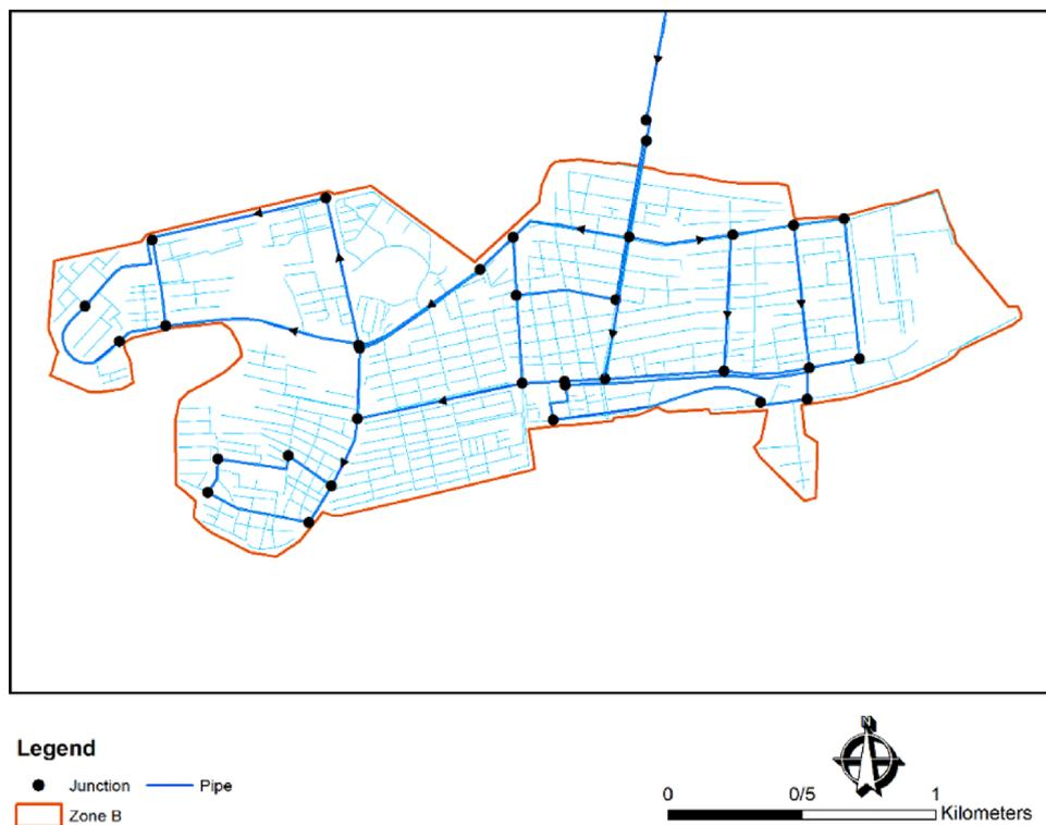
**Figure 7.** Zone B of Birjand water distribution network modeled in WaterGEMS software.
