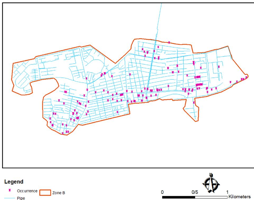
**Figure 8.** The density of failures in zone B of Birjand WDN in Iran.
