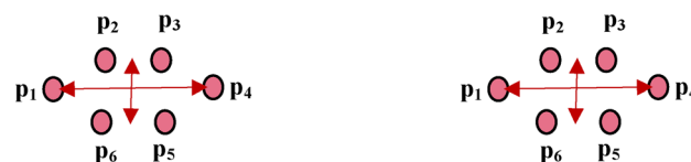
Figure 4. The 6-coordinates of left and right eyes, which are used in the Eye Aspect Ratio, EAR, computation.
