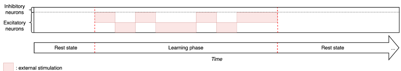
Figure 2. Diagram representing the stimulation protocol divided in three phases: a first short phase of spontaneous activity, a learning phase during which two different groups of excitatory neurons are stimulated alternately over time (the red areas represent the duration and the neurons that received external stimulation), and a final long period of resting-state activity in which the plasticity remains active.
