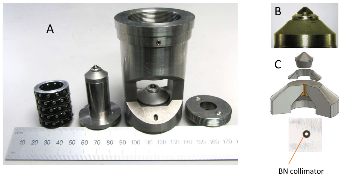
Figure 1. Megabar neutron diamond anvil cell. (a) A photo of the individual parts of the cell, roller bearings, top piston including seat and anvil, cell body including opposing seat and anvil, and top closing cap. (b) A photo of the seat and anvil including the steel binding ring used for additional support. (c) A 3D-schematic created in Autodesk Fusion 360 (V2.0.15050, https://www.autodesk.com/products/fusion-360 ) of seat and anvil including the collimator built into the seat consisting of amorphous boron with a small amount of epoxy. A close-up photo of the seat in top-view shows the aperture for incoming beam formed by the collimator. The diameter of the hole in the seat is thereby 1 mm diameter.
