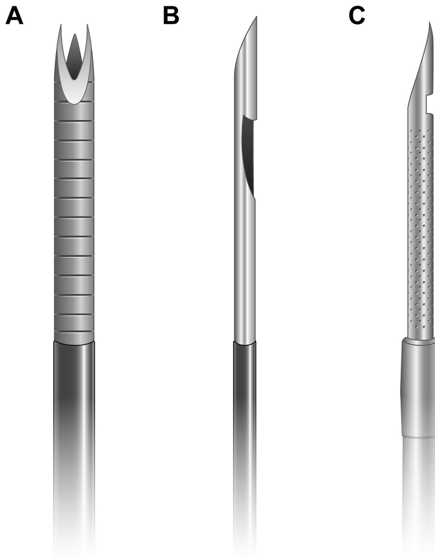
Figure 1. (A) The Franseen needle has a novel design of a crown tip with three-plane symmetric cutting edges. (B) The Reverse-bevel needle has a reversed-bevel system as a side-fenestrated opening on the needle shaft. (C) The Menghini-tip needle has a tapered bevel edge that facilitates the tissue being withdrawn into the lumen. Although it has a side port, it is classified as FNA needles because the side port of this needle system does not have any reinforcement geometries for cutting the tissue.
