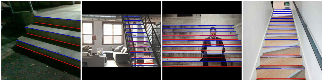
Figure 1. Illustration of the difficulties encountered in stair detection. The convex lines are marked with blue, and the concave lines are marked with red. The figure shows some challenging scenarios, including extreme lighting conditions, special structures, severe occlusions and special materials.
