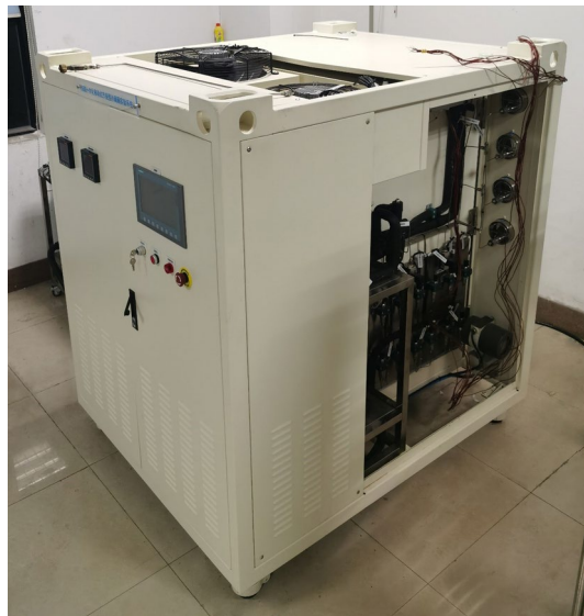
Figure 3. CO 2 transcritical refrigeration experimental platform.
