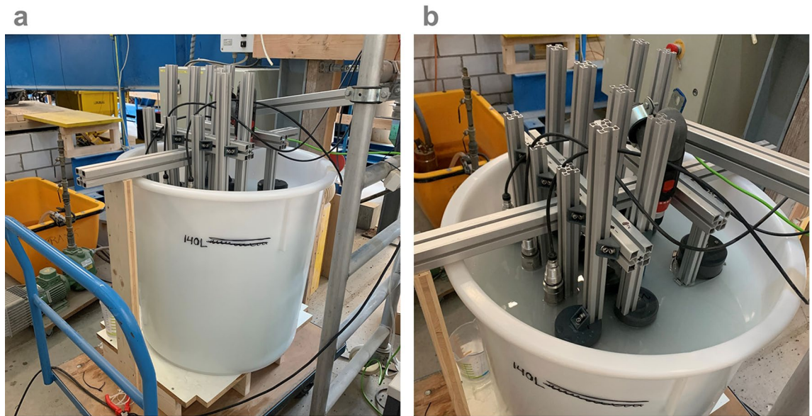
Figure 10. Mixing tank setup: (a) cylindrical 200L tank, (b) arrangement of 11 sensors (8 of ours and 3 commercial) within the tank and the mixing drill in the middle.
