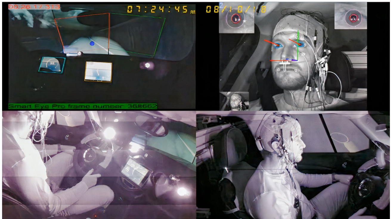
Figure 1. Four different views of the driver when he was conducting the test. The test road in a night drive and a dashboard instrument that shows the velocity of the vehicle in the simulated test track are shown in the left part. The output of the eye-tracking system that detects the eyelid movements and pupil diameter is presented in the right upper part (Reprinted from our previous study 14 ; Copyright (2021), with permission from Elsevier, License No. 5058681457961. Informed consent was obtained from the driver to publish his image.
