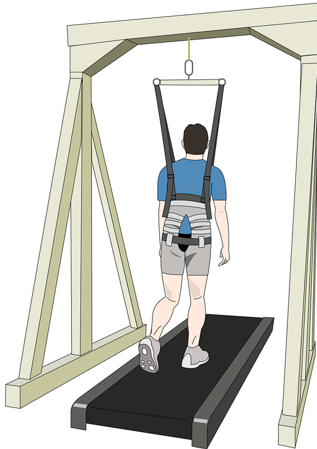
Figure 1. Reduced gravity simulator during walking. Participants walked on a treadmill while a body weight support system vertically pulled up on the participants' torsos using a harness attached to their thighs and waist to reduce the load on supporting legs corresponding to 0, 40, 62, 84, or 93% of their body weights. This figure was created by one of the authors of this paper, Shota Hagio, using Adobe Illustrator 2020 (Adobe Inc., San Jose, CA, USA; https://www.adobe.com/jp/products/illustrator.html ).
