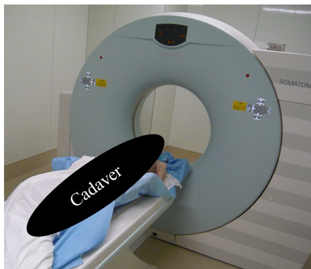
Figure 3. SOMATOM Emotion 16-slice computed tomography scanner (SIEMENS) installed in the cadaver research institution.
