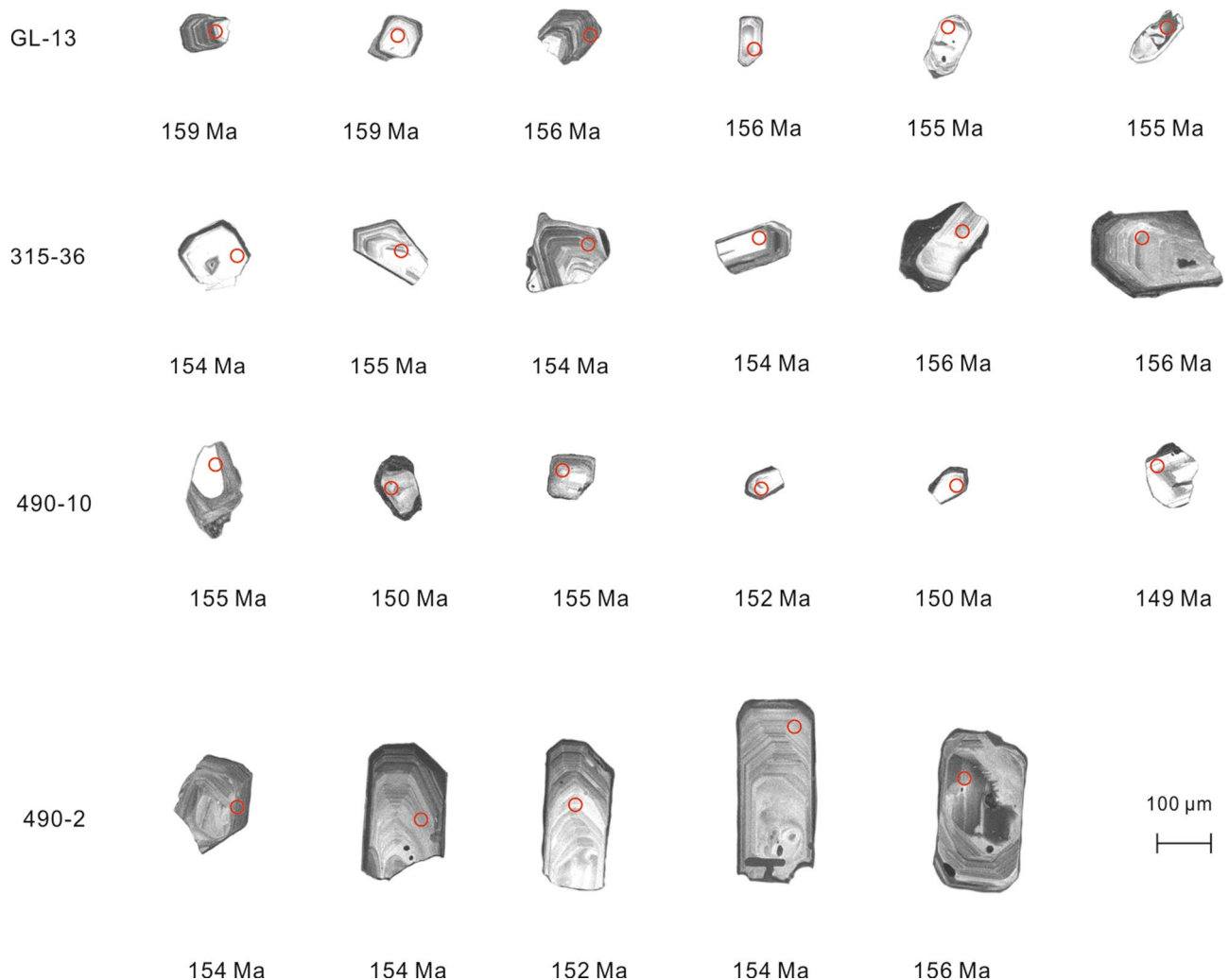
Figure 5. Cathodoluminescence images of zircons with corresponding ^{206}\text{Pb}/^{238}\text{U} ages for the samples from the QGC.
