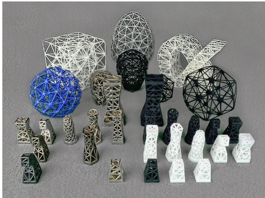
Figure 5. A menagerie of AM-printed Hgon structures with wide-ranging simple and complex shapes. Several materials and processes are shown including SLS (sintered) alloys of steel, bronze, brass, aluminum, titanium and plastics e.g. nylon and ABS, Jet-fusion, and SLA printed resin. See the “Appendix” for further information and 3D-VR views of these and other meta-structures.
