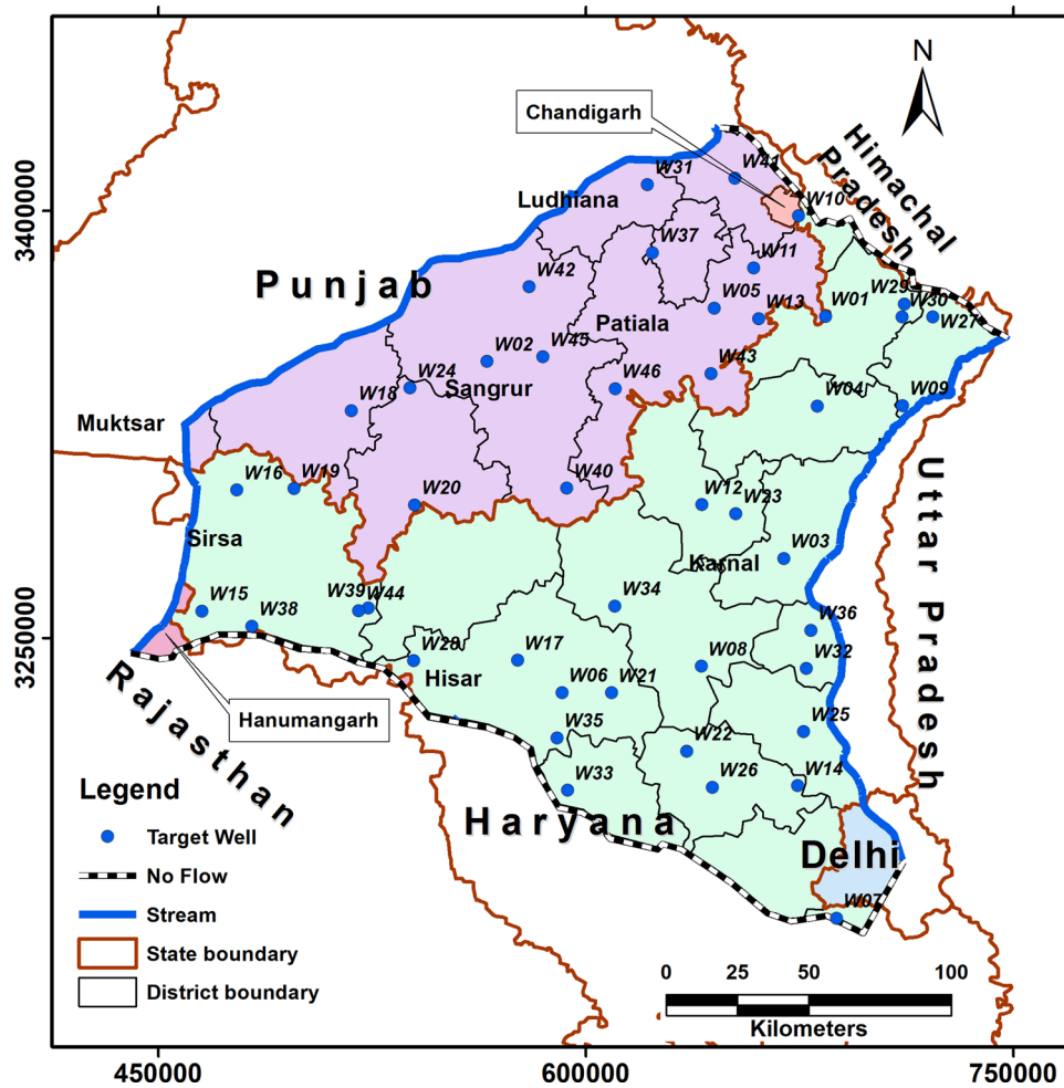
Figure 4. Map showing the model boundaries and the location of the 46 CGWB target/observation wells used in the model calibration and validation.
