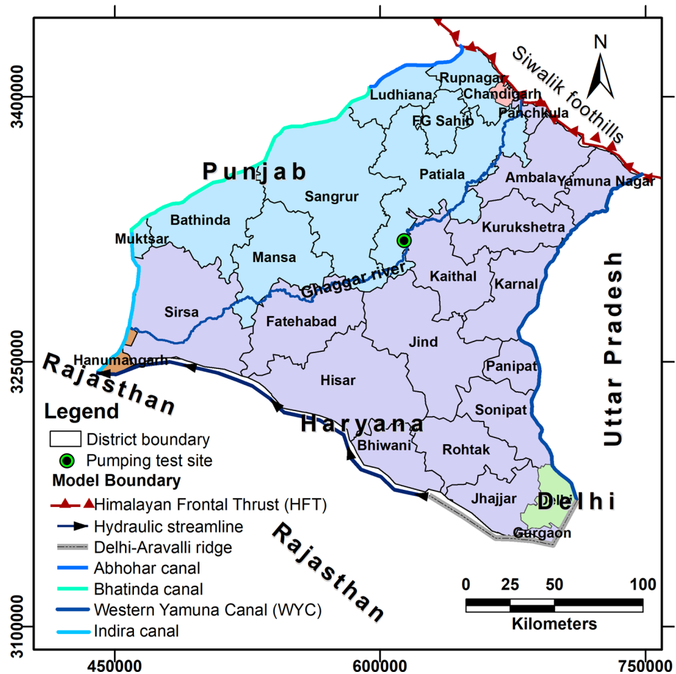
Figure 2. Map showing the model area with district names and model boundaries (Himalayan Frontal Thrust; hydraulic streamline; Delhi Aravalli bedrock ridge; various canals) and the pumping test site in Patiala district.
