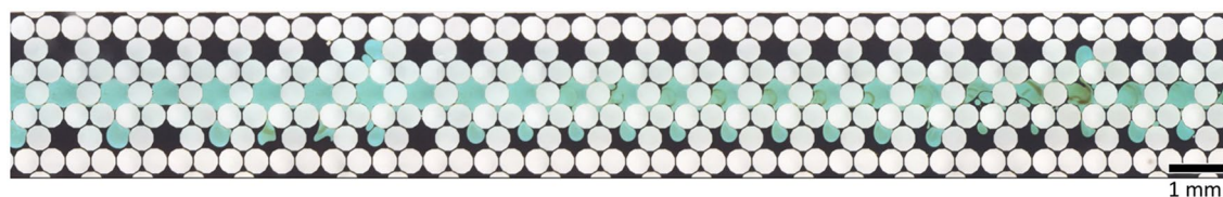
Figure 8. Representative image of micromodel state at the end of water flooding. Dark brown pores are oil-filled while blue/green pores are water filled. The light brown color in the water-filled pores indicates the presence of an oil film.
