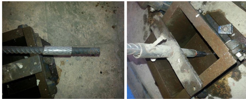
Figure 6. Moulds and testing cubes with steel rods inserted.
