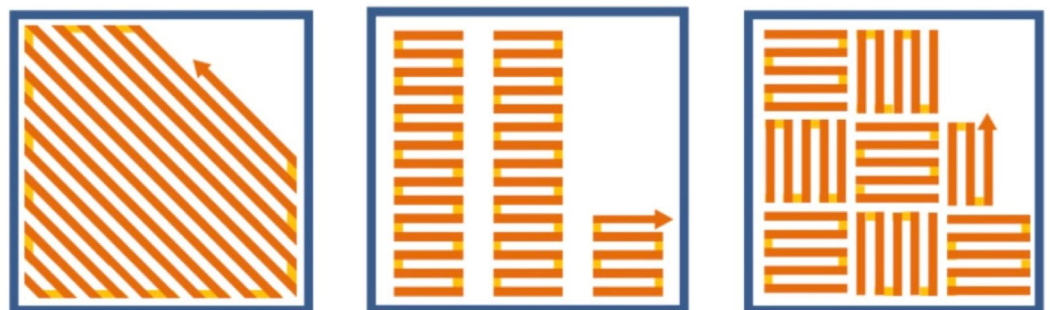
Figure 16. Schematic illustration showing the laser scanning strategies used in the current study, (a) Meander; (b) Stripes; (c) Chessboard.
