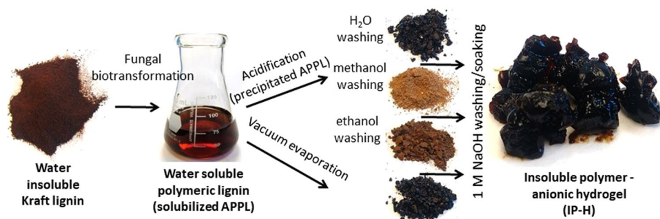
Figure 7. Graphical Abstract: Production of lignin based insoluble polymers (anionic hydrogels) by C. versicolor
