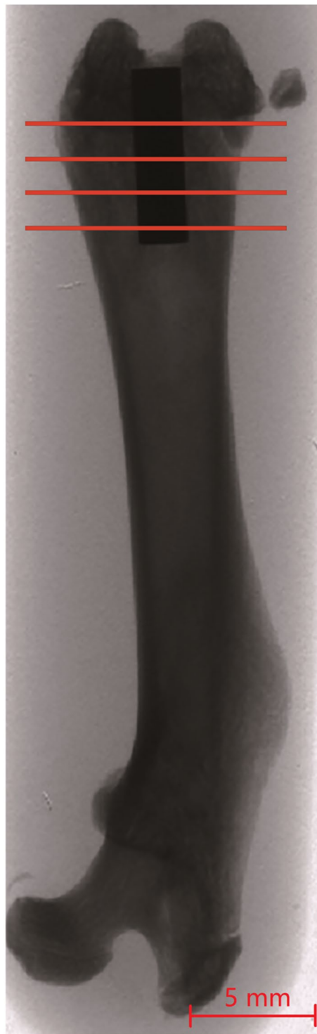
Figure 6. Radiographs indicating the position of the implant within a rat femur. The lines illustrate the four cutting levels. Scale bar, 5 mm.
