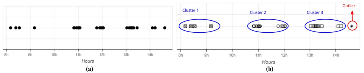
Fig. 5 Distribution over time of interaction sequences (a) Distribution over time of interaction sequences from a single operator. (b) Identified clusters after applying Meanshift Algorithm for time interval detection.
