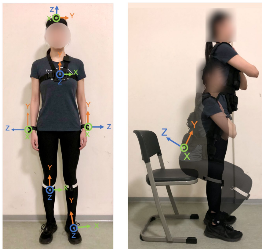
Fig. 2 Experimental setup. Left: sensor placements and orientations. Right: sit-to-stand fatigue protocol.
