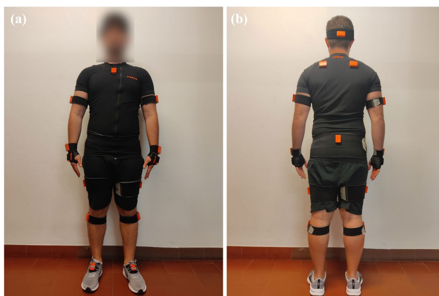
Fig. 1 Inertial sensors placement: (a) participant's anterior view, and (b) participant's posterior view. Note that each sensor was placed in the inner of the strap to better secure the sensors. Additionally, the sternum , head, and foot sensors were placed inside the frontal pocket of the Xsens suit, on the pocket of the headband and inside each shoe, respectively.
