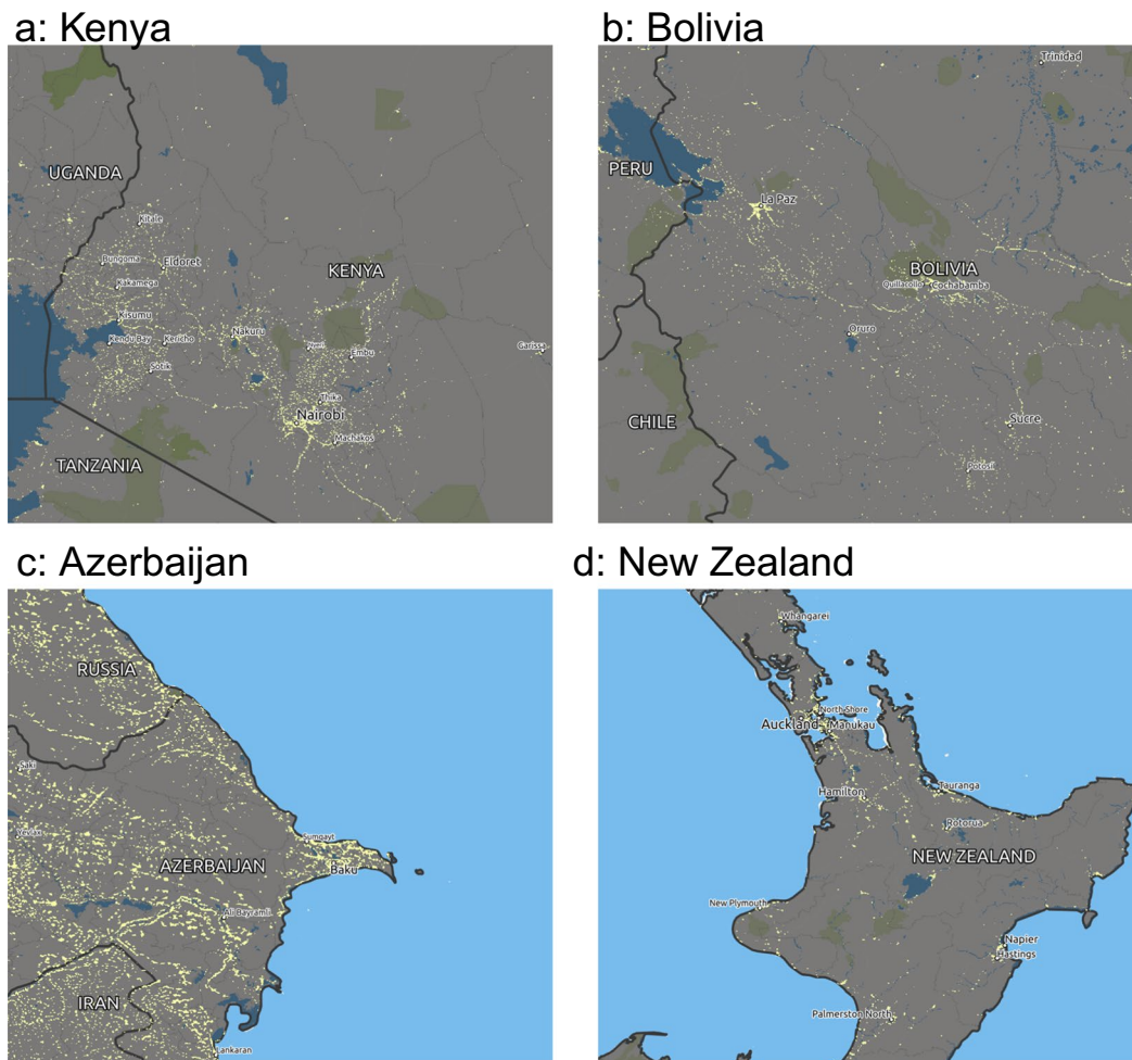
Fig. 2 Night-time lights as a proxy for electricity access in four countries with different income levels. (a) Kenya, low-income but regions of dense light-emission; (b) Bolivia, lower-middle income; (c) Azerbaijan, higher-middle income and dense population; (d) New Zealand's North Island, high-income but largely rural. This data can also be visualized interactively here: https://gridfinder.org .
