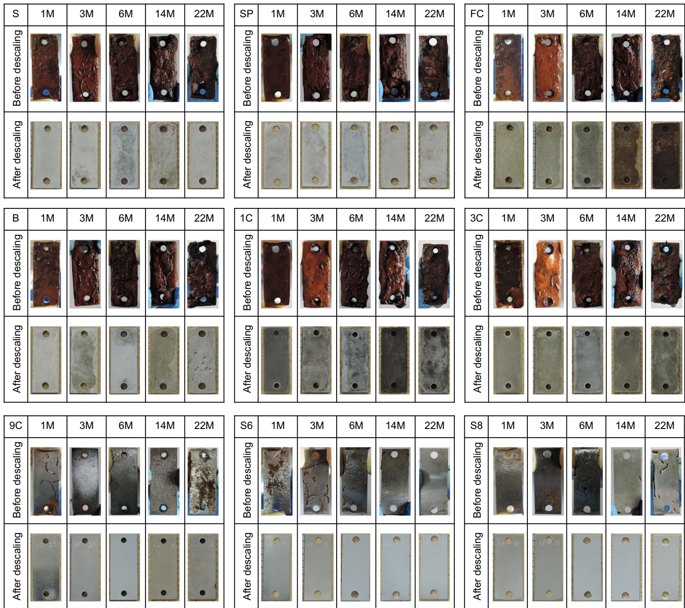
Fig. 1 Coupons after immersion study. Macroscopic images of each coupon (50 mm high × 20 mm wide) are shown before and after descaling. 1 M, 1 mo; 3 M, 3 mo; 6 M, 6 mo; 14 M, 14 mo; 22 M, 22 mo; S, ASTM A283; SP, ASTM A109 Temper 4/5; FC, ASTM A395; B, ASTM A179; 1 C, 1% Cr steel; 3 C, 2.25% Cr steel; 9 C, 9% Cr steel; S6, type-316 stainless steel; S8, type-304 stainless steel.
