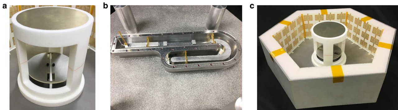
Fig. 3 The fabricated A-SBFA. a Fabricated slotted patch feed and subreflector with 3D-printed mounting fixture. Both were machined out of aluminum. b Underside of A-SBFA, showing fabricated impedance matching network. c View of assembled A-SBFA showing 3D-printed aluminum cavity, feed antenna and subreflector, as well as copper metasurfaces etched on a thin substrate and separated from cavity walls by a low permittivity foam layer
