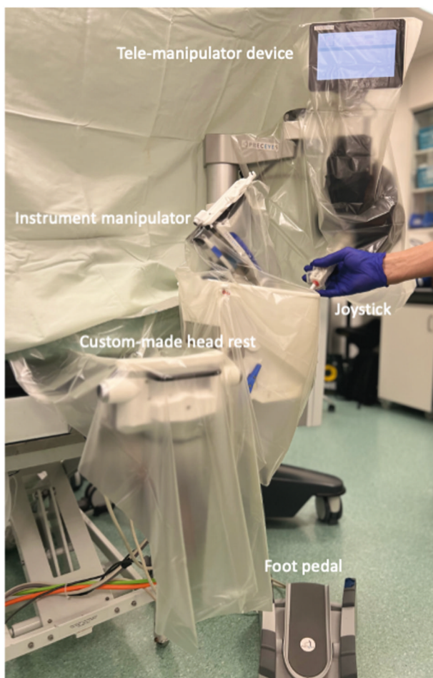
Fig. 1 The Robotic System in clinical use: The Preceyes Robotic Surgical System (Preceyes BV). The system work as a telemanipulator device with separate joystick and manipulator.
