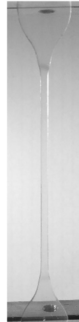
Fig. 10 Photograph of LMPP under 1.00 strain
