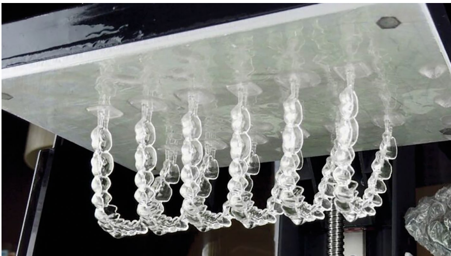
Fig. 3 Graphy direct aligner printing. Image reproduced with permission from Graphy Inc ( http://itgraphy.com )
