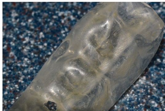
Fig. 8 Marked wear and crazing of acrylic
