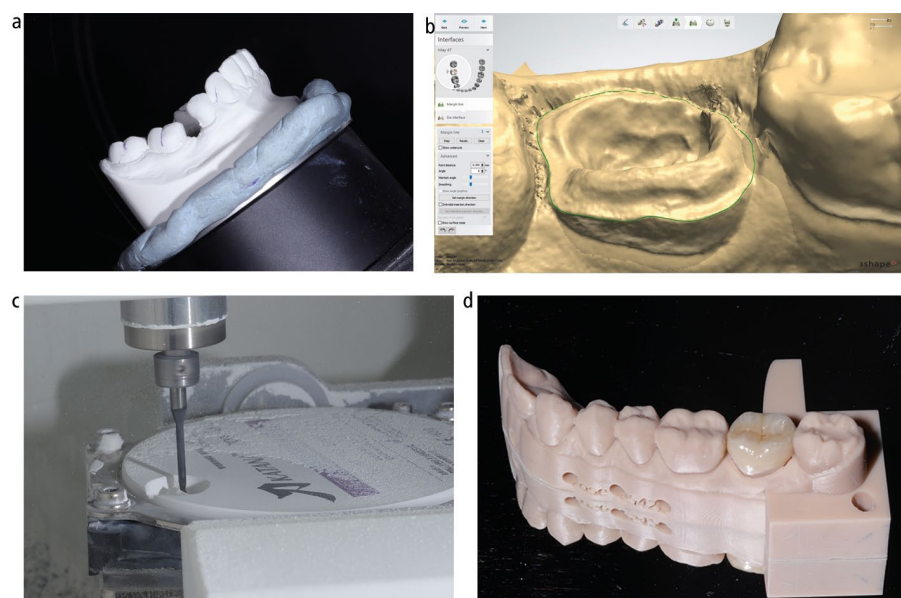
Fig. 4 CAD/CAM. a) Scanning of model. b) Design of restoration. c) Dry milling of zirconium. d) Final restoration
