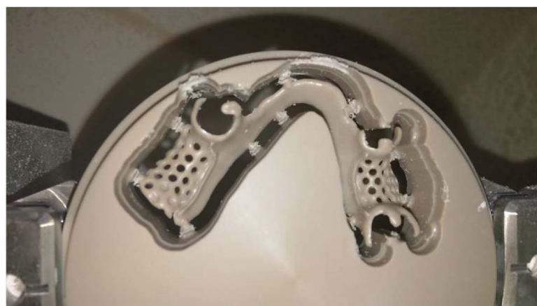
Fig. 4 RPD milled from AKP showing the attachment points between the framework and AKP block
