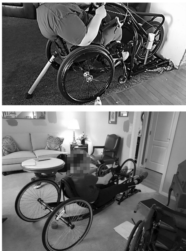
Fig. 1 Example HIIT training setups used in the study. The top figure shows the add-on handbike setup. The bottom figure shows the full handcycle setup.
