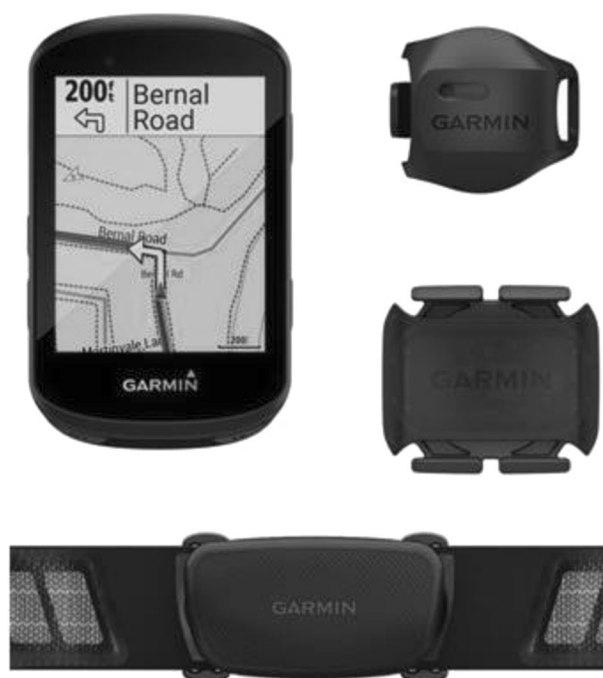
Fig. 2 The Garmin 520 bike computer and sensors used in the study.
