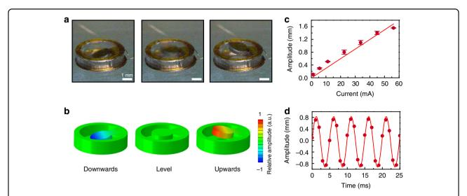
Fig. 3 Vibration behaviors of actuators with a resonance frequency of 200 Hz. a, b Optical images captured using a high-speed camera (a) and FEA results (b) of the actuator traveling in a downward direction (left columns), leveled, and traveling in an upward direction. c Relationship between actuator amplitude and input peak sinewave current. d Values of the vibration amplitude with time
