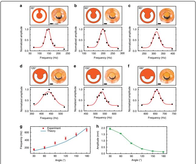
**Fig. 2 Optimization of frequency and amplitude of the vibrotactile mini actuators. a–f** PI discs with different central angles ranging from 30° to 180° (top row, left), top views of the corresponding actuators (top row, right), and normalized amplitude–frequency responses of actuators (bottom row). **g** Dependence of the resonance frequency on the central angle. **h** Amplitude changes of the actuators at the resonance frequency with the central angle
