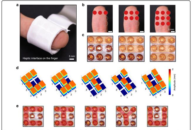
**Fig. 4 Programmable control and pattern actuation of e-skin for a haptic interface. a** Photograph of e-skin on a finger. **b, c** Subregional control of the e-skin. Optical images of the corresponding finger area (**b**) and actuated area of the array (**c**). **d, e** Programmable actuation of the e-skin in a "CITYU" pattern. Amplitude distributions (**d**) and optical images of the programmed actuation area (**e**)
