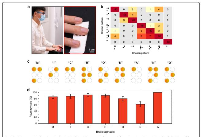
Fig. 5 Braille recognition based on the haptic interface. a Photograph of the tester's finger placed on the haptic interface. b Grid view of the test results. c Braille letters "MICRO-NANO" and the corresponding actuator positions. d Testing accuracy rate for braille letters "M, I, C, R, O, N, A"
