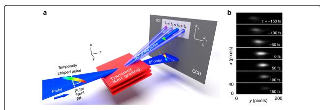
**Fig. 4 Visualization of angular dispersion. a** Concept of the diffraction of an angularly dispersed probe pulse by the transient grating. The transient grating effectively samples the chirped pulse at the pump–probe delay and diffracts the corresponding sub-pulse on the ROI (region of interest) in the first order of diffraction. **b** Typical experimental result. Diffracted signal as a function of delay and deviation angle in y direction.
