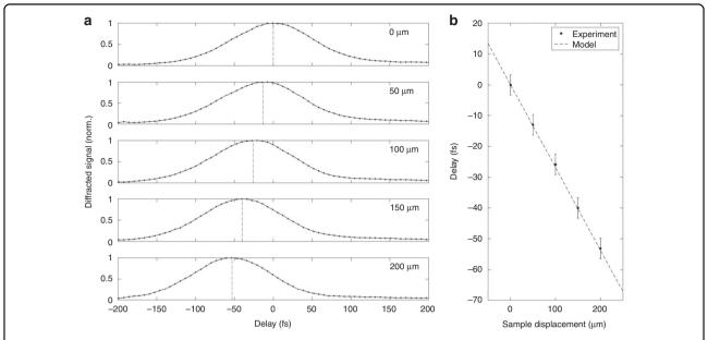
**Fig. 3 Pump-probe delay change by sample translation. a** Evolution of the TG signal as a function of sample position in sapphire (from 0 to 200 μm). **b** Barycenter of TG signal as a function of sample displacement; experimental data are in excellent agreement with the model of Eq. (2). The parameters are provided in the "Methods" section. The error bar is due to the determination accuracy of the barycenter, linked to the positioning accuracy of the delay line.
