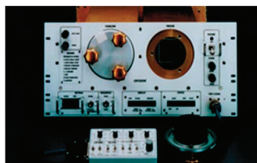
Figure 4. Cryostat crystallization flight hardware. This hardware was built by DARA, the German Space Agency, and provided fourteen crystal chambers maintained at controlled temperatures.
