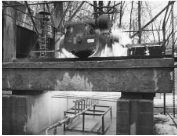
Fig. 2. Fire-resistance testing of ball cock ( D_n = 400 mm, and p_{\text{eff}} = 8 MPa) produced by Tyazhpromarmatura (heat-insulating housing is removed).
