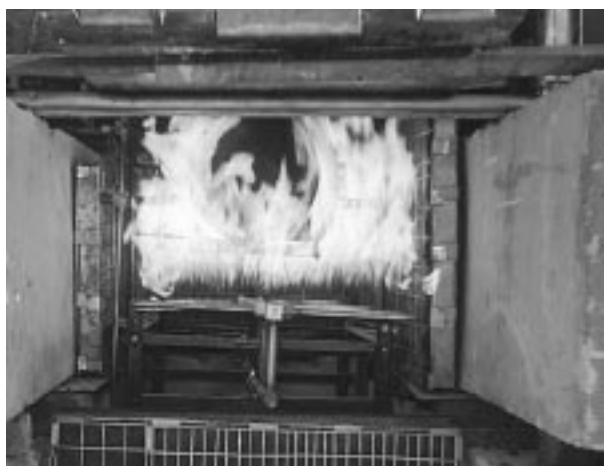
Fig. 3. Fire-resistance test of vehicular cylinder produced by the KMZ (ambient temperature of -15^{\circ}\text{C} ).
