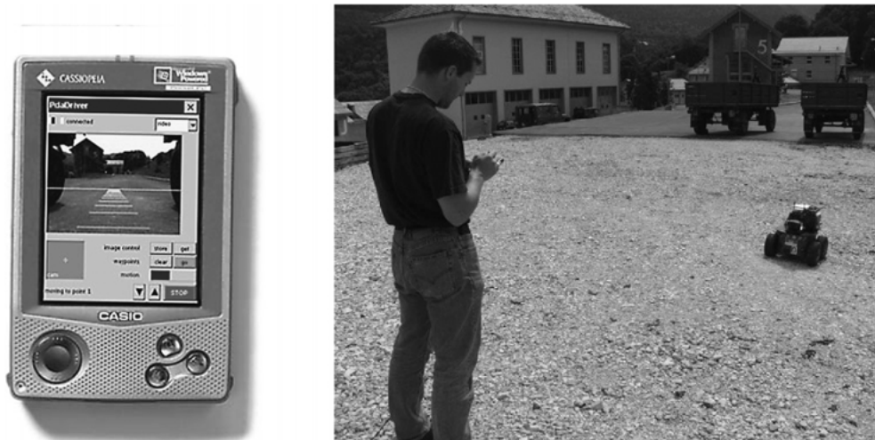
Figure 12. PdaDriver is a Personal Digital Assistant based interface for remote driving (Carnegie Mellon University and Swiss Federal Institute of Technology, Lausanne).
