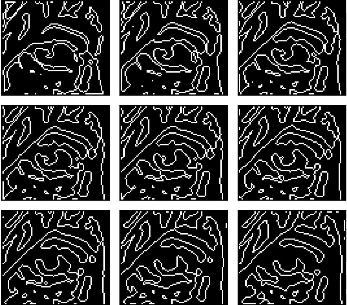
Figure 8. Pseudo-linear Laplacean zero-crossings, \Delta v + \mu \|\nabla v\|^2 = 0 , computed for the image shown in Fig. 7. First and second derivatives have been computed as linear scale-space derivatives at an arbitrarily chosen scale \sigma = 2 pixels, i.e. by convolution using corresponding derivatives of a normalised Gaussian of width \sigma = 2 . The original image has been normalised to the unit interval prior to edge detection. From top left to bottom right we have parameter values \mu = -8, -4, -2, -1, 0, 1, 2, 4, 8 , respectively. Observe how the topology of the zero-crossings changes with \mu .
